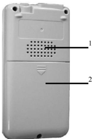
**Fig 1-2 Rear view of the oximeter**
