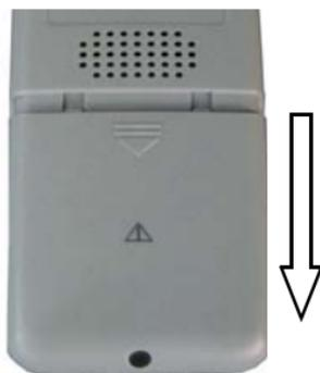
**Fig 7-2 Push the battery door**
