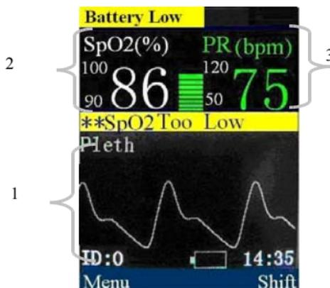
Fig 1-5 SpO<sub>2</sub> waveform display mode
