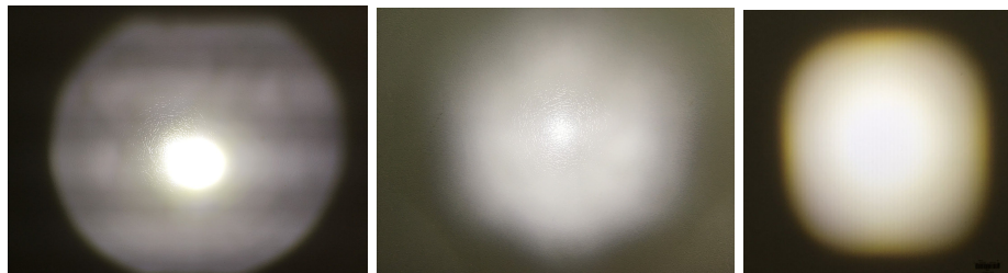
Figure 4.24: Headlight lighting uniformity comparison. From left to right: recreational headlamp using a reflector; recreational headlamp using a gross fresnel lens and diffuser; surgical headlamp using a fine fresnel lens.
